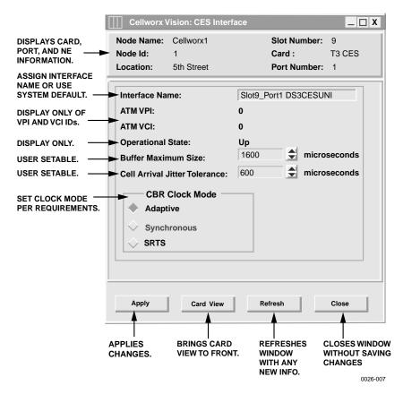
Figure 792-2. T3 CES Interface Configuration Screen
